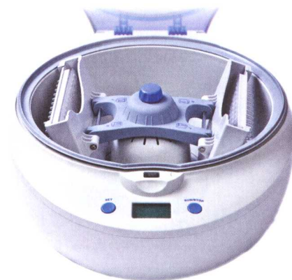
Fig. 8: The interior of the FastGene® Plate Centrifuge
